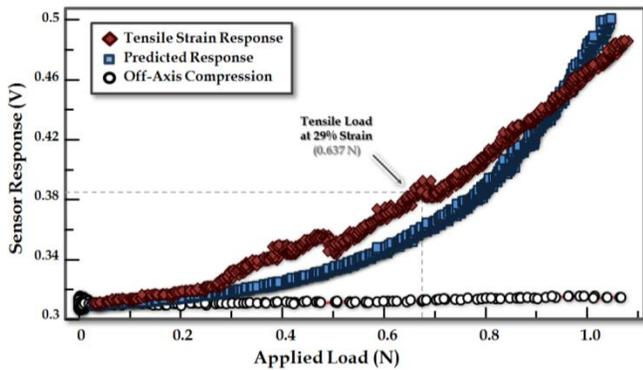
Fig. 6. Response of a strain sensor 1cm in width and 2mm in thickness with a  $h = 500\mu\text{m}$ ,  $w = 300\mu\text{m}$ , and  $L = 97\text{mm}$ . Resistance changes were recorded using a voltage divider with a 1V source and 10 Ohm reference.
