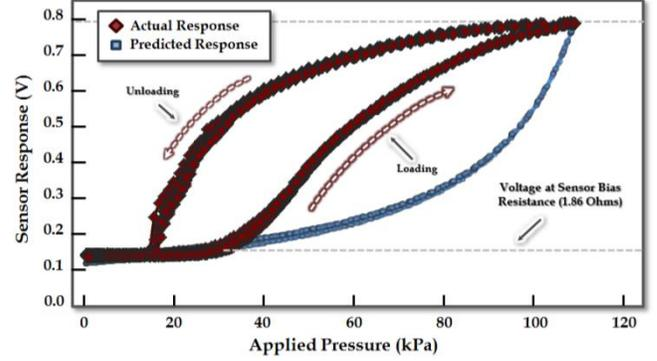
Fig. 4. Response of a pressure sensor 1cm in diameter and 2mm in thickness with  $h = 500\mu$ m,  $w = 300\mu$ m, and  $L = 157.4$ mm. Resistance changes were recorded using a voltage divider with a 1V source and 10 Ohm reference.
