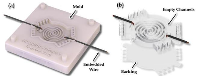
Fig. 8. Soft sensor fabrication process innovations in this work include (a) placement of embedded sensor components into mold before (b) silicone casting and curing.
