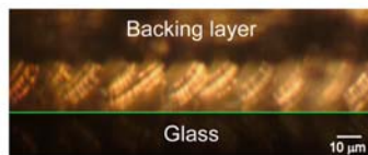
Figure 7. (a) Resulting friction forces for experiments where constant compressive displacement or force is applied to fiber arrays or flat surfaces by a sliding glass hemisphere. Error bars represent the standard deviation for the five trials at each data point. (b) The sidewall contacts of the fibers seen under optical microscope.
